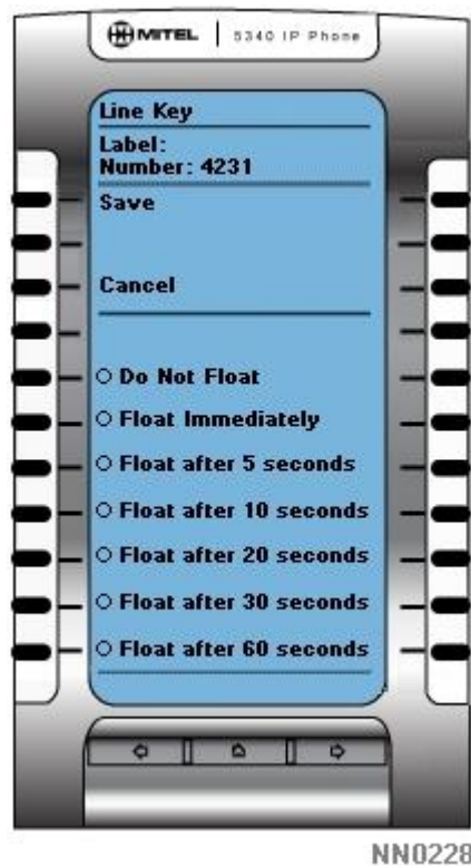
Figure 3 5340 Float Key Configuration Window
